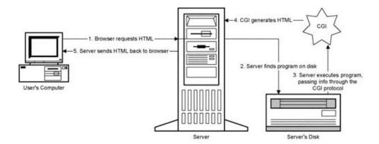
Figure 1.2. How a server generates dynamic content.
