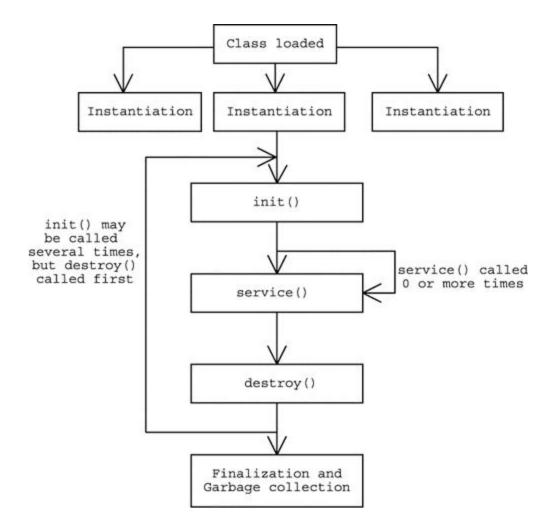
Figure 11.1. The servlet life cycle.
