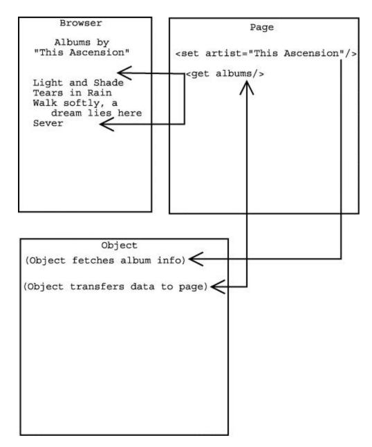
Figure 1.6. A tag that uses an object.
